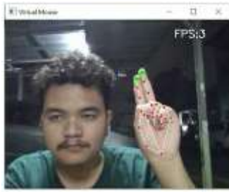
Gambar 11. Hasil deteksi landmark scroll down
