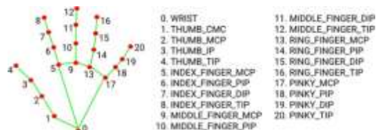
Gambar 1. Hand Landmark MediaPipe Model
